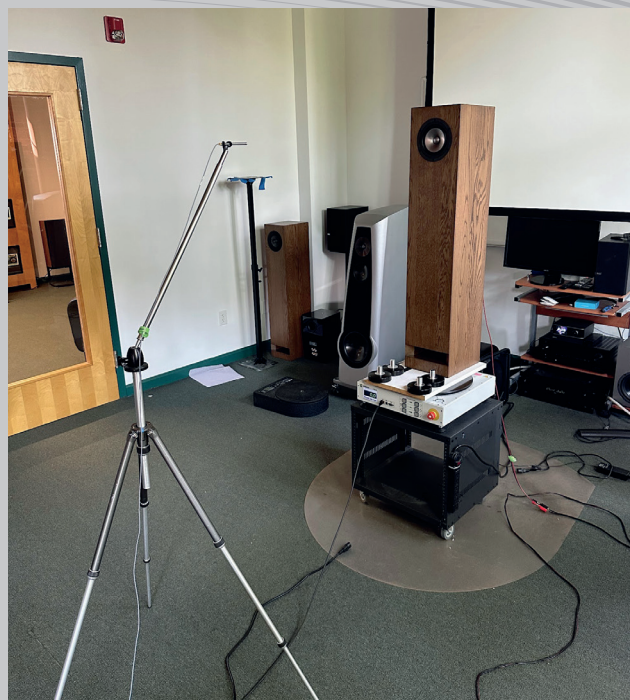
Measurement setup: the Pearl Acoustics Model One on the measurement turntable, with the measurement microphone 1m from the driver.
